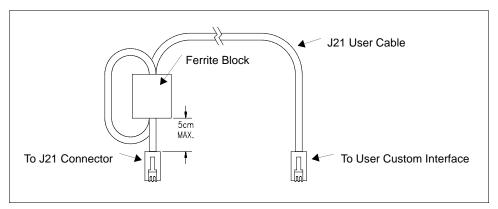
Figure 2.6 J21 User Cable with Ferrite Block
