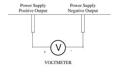
Figure 4.1 Voltage Calibration Setup
