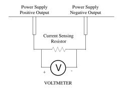
Figure 4.2 Current Calibration Setup
