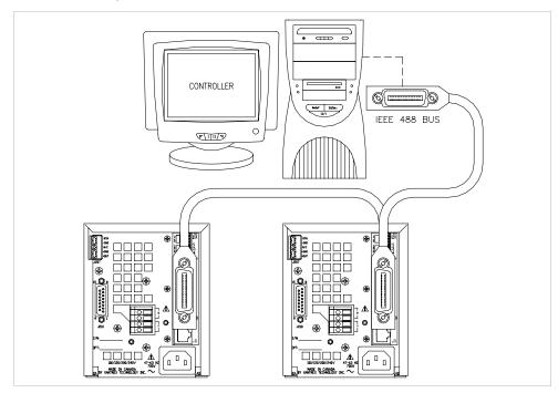
Figure 1.1 Sample Configuration using GPIB Interface
