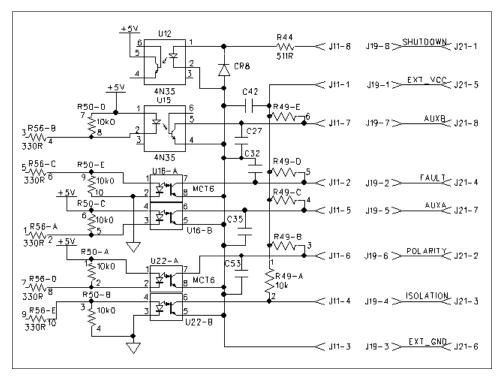
Figure 2.5 J21 User Signal Connector Circuit Block Diagram
